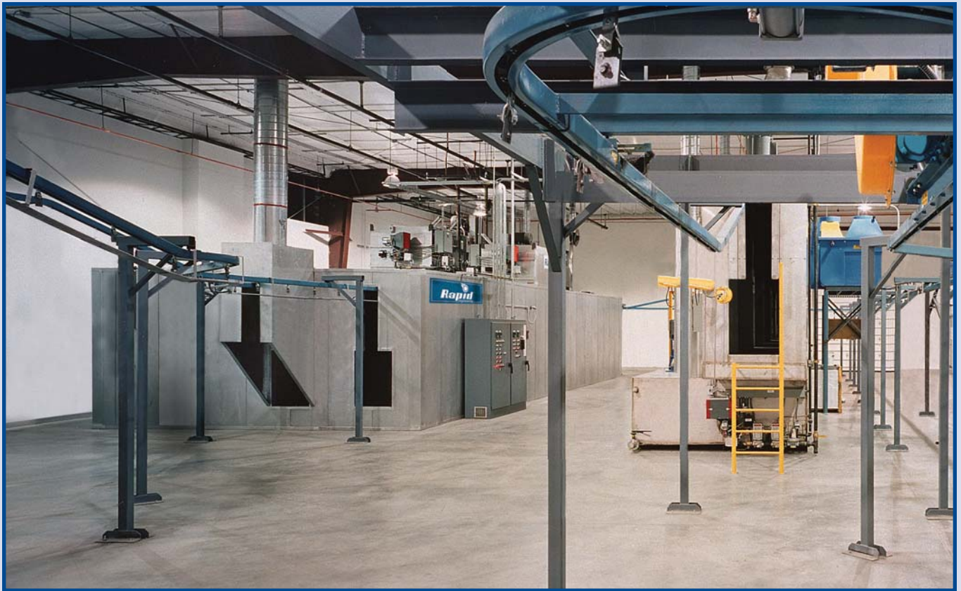
A typical RAPID® finishing system with five-stage washer, dry-off oven, cure oven, conveyor and controls.
