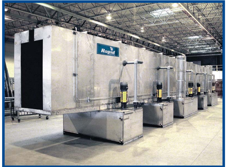
The RAPID® Econo series multi-stage washer was specifically designed to meet common manufacturing product sizes and required production throughput from 4 to 8 feet per minute.
