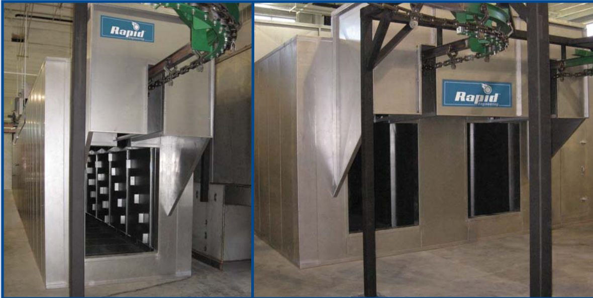
RAPID™ Dry-Off Oven and Cure Oven.
