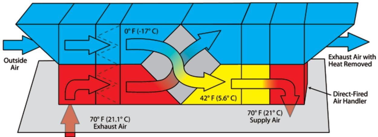
Figure 2 Once the heat exchanger is incorporated into an enclosure, the energy-recovery module can then be mated with supply and exhaust fans for the two air streams. A common application is depicted here.
