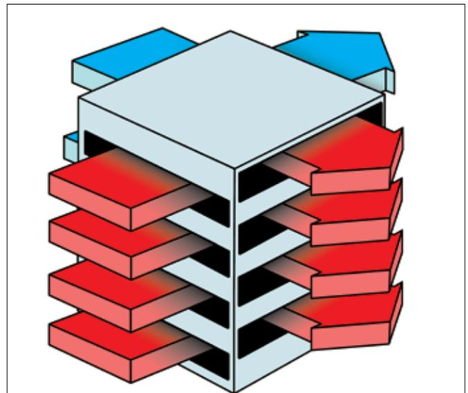
Figure 1 This illustration depicts the perpendicular air flow from one layer to another in a fixed-plate heat exchanger.
