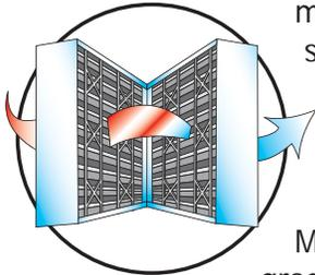
Most systems will have commercial grade 30% filters as the first level of filtration in the process. These filters remove the larger particles and help extend the life of the more costly final filters. These filters are 30% efficient on a 1 micron particle, and are designed to be changed monthly.
